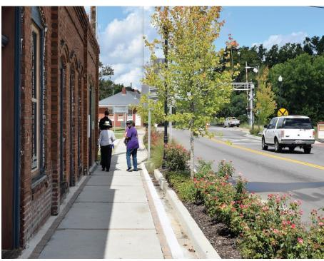
Sidewalks: The primary purpose of sidewalks is to provide a safe path for pedestrians that is separated from vehicular traffic by on-street parking or a planting strip. Width of sidewalks should be a minimum of 5 feet in low density residential areas and increase in width in areas of high pedestrian traffic. Sidewalks should be prioritized where they provide safe and convenient access for pedestrians to schools, parks, retail, and services.
